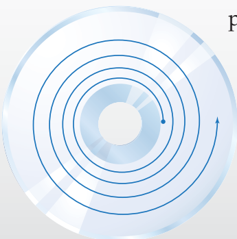
The laser from a player reads the disc from the inside out.
