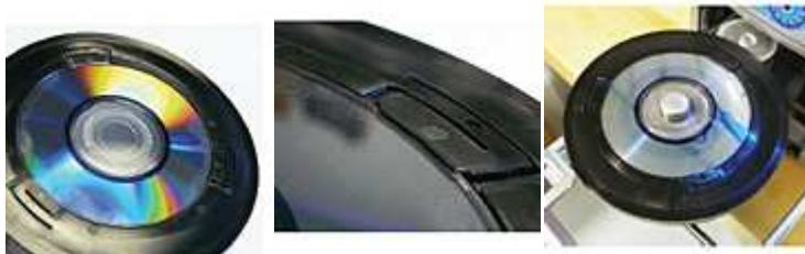
Match the label side of your 3 inch disc with the open side of your 3 inch adapter. Slide the disc into the 3 inner grooves making sure that the disc is firmly clipped in place. The optical side should be facing you.
