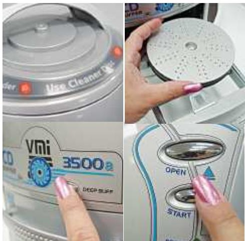
The VMI 3550i will indicate when it is time to run a cleaning cycle for the buffing wheels. After 15 cycles the USE CLEANER DISC lights will flash indicating that after the next cycle the cleaner disc should be used. After the 16th cycle, the USE CLEANER DISC lights will flash, and the unit will sound a tone, indicating that a cleaning cycle should be run.
