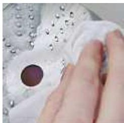
The VMI Cleaner Disc must be maintained on a regular basis. You can identify that the Cleaner Disc needs cleaning, by seeing a heavy build up on the surface.
