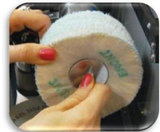
6. Remove the screw and the washer from the spindle and pull off the old Buffing Wheel.
