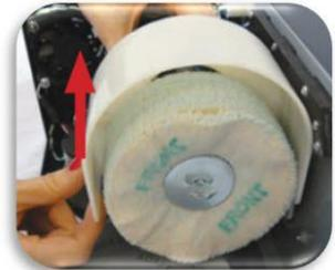
5. Located on front of the Buffing Wheel, is a washer and a Spade style screw, which holds the Buffing Wheel to the spindle. Hold the Buffing Wheel with one hand and turn the Spade Screw counter clockwise with the other.
