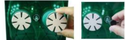
Installing the Pads and Centre Hub
